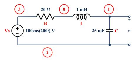
the following LTspice netlist can be used to determine the magnitude and phase angle of the steady-state AC part of v:
